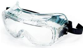
Clear UV-absorbing polycarbonate lens. Soft, clear goggle body. Indirect vents top and bottom. Fits over most prescription eyewear. Meets ANSI Z87.1-2003 Standards. CUL Certified to meet CAN/CSA-Z94.3 Standards.
